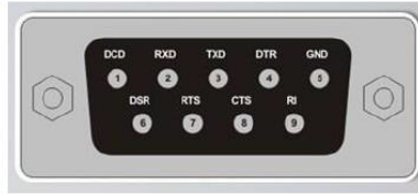
Fig 2-9 DB9 hole definition
